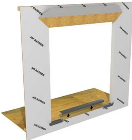
Figure 12: Install center piece and apply adhesive
